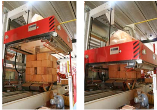
Hooder with Hot Air Thermoshrinking Device
