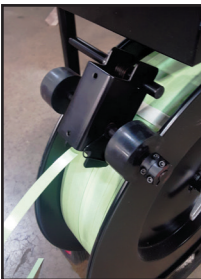
EXTRA HEAVY DUTY REEL BRAKE PREVENTS STRAP TANGLES RESULTING FROM THE COIL OVER SPINNING
