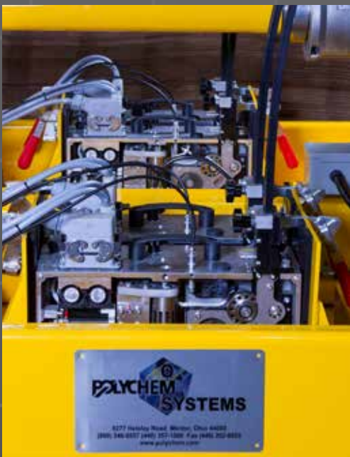
TOP OF PLATEN VIEW SHOWING 4 SX600 ULTRASONIC HEADS
