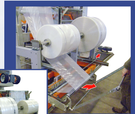
PORTABOBINA ESTRAIBILE EXTRACTABLE COIL HOLDER
