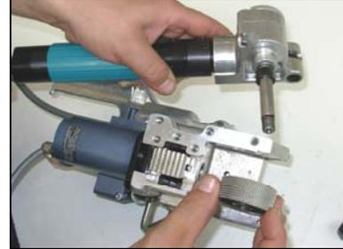
Remove the pushing spring (pic.M1), disconnect the motor pipe (pic.M2), remove the 6 bottom plate screws (pic.M3), unscrew the holding screw (pic.M4), remove the nut on connection shaft (pic.M5) and pull it out from main frame (pic.M6) pay attention to the shim. Remove the feed wheel shaft nut (pic.M7) Remove the front cover, the bush, the clutch system with the feed wheel (pic.M8); replace the worn part (pic. M9) Reassemble in reverse order.
