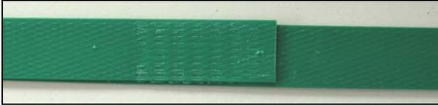
**NO** – seal strength insufficient
