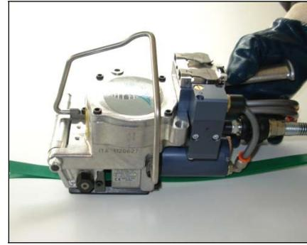
Push the tension lever #1(pic. D4) until desired tension is reached or until the motor stalls. Release lever #1 and push lever #2 one time (pic. D5) to cut and weld the strap. (Adjust time before sealing).Welding and cooling time will be signalled by the little piston (pic. D6) when piston returns the welding cycle is complete (pic.D7). At this point you can remove the strap by following the instructions below.
