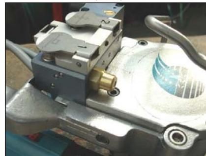
**WARNING: Wait until the piston returns (pic.D7) before releasing the strap**
