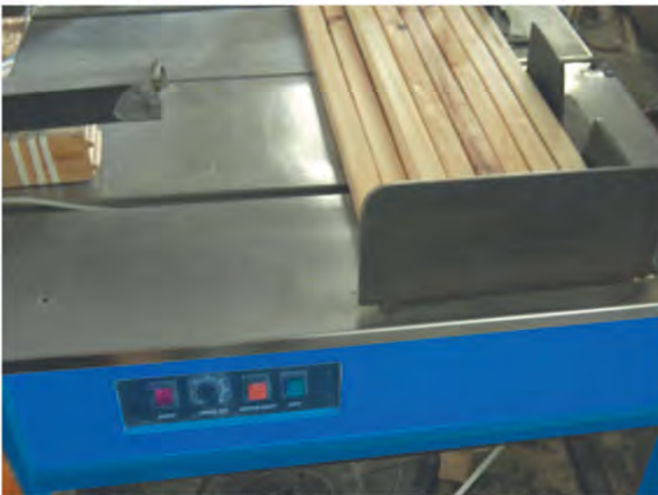
Polychem's PC 102's are excellent for bundling lighter weight loads like spindles and balusters
