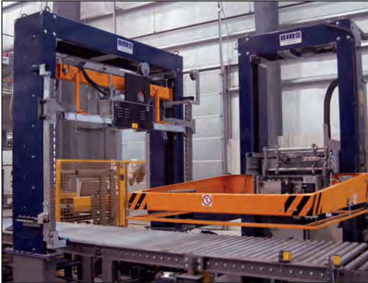
OMS Paver System with Vertical and Horizontal Strappers
