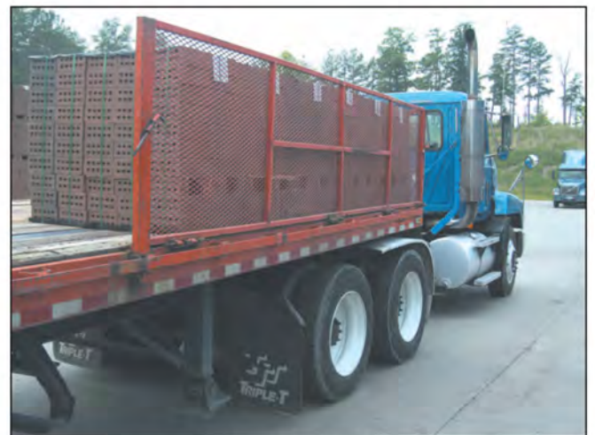
Another truck load of polyester strapped brick moving out.
